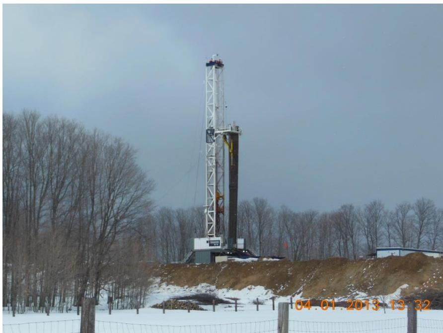
The permit issued by the Michigan Department of Environmental Quality authorized one water well on the site. The estimated water required for the gas/oil well was 8.4 million gallons. (That compares to about 10,000 gallons used to complete or “stimulate” wells in the traditional way – a massive increase in consumptive water use by the fracking industry compared to the past.)
